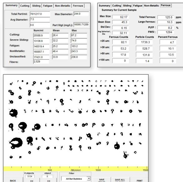
Wear images are stored and analyzed directly on the LaserNet 200 software. They can be sorted by wear class. OilView™ software also reports on particle count and size distribution by wear category.
