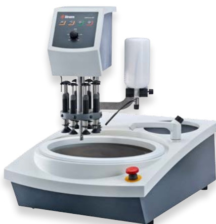
LaboForce-Mi is a semi-automatic specimen mover for the production of thin sections, polished thin sections and polished specimens of mineralogical materials. The force is applied through springs which can be individually adjusted
