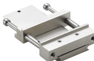
Specimen holder CATSI, for general use Max. opening: 60 mm. To be used with a fixed stand, manual X-stand, or a rotary stand.
